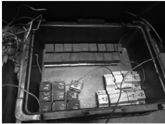
图 2 碳滑块试块 Fig.2 Carbon contact strips test block sample
