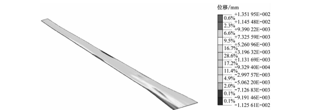
图 4 工况一水平位移云图 Fig. 4 Nephogram of horizontal displacement under working condition I
