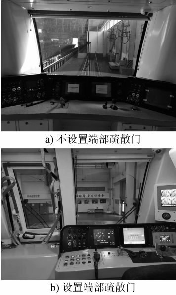
图 2 端部疏散门对司机室布局的影响对比照片 Fig. 2 Comparison pictures of influence of end evacuation door on driver's cabin layout
