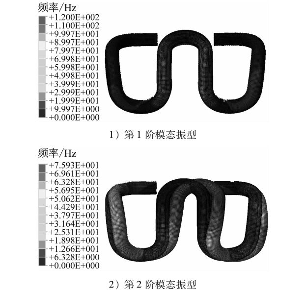
图 5 WJ-2 型弹条在标准安装状态下的前两阶模态振型 Fig.5 The first two order mode shapes of WJ-2 type elastic rod in standard installation state
