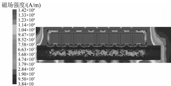
图 11 励磁电流为 95 A 时涡流制动系统磁场分布云图(紧急制动工况) Fig. 11 Nephogram of eddy current braking system magnetic field distribution with excitation current of 95 A (urgent braking condition)
