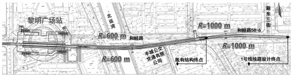
图 4 既有沈阳地铁 1 号线终点站及站后区间方案截图 Fig. 4 Screenshot of the terminal station and interval behind station of existing Shenyang Metro Line 1
