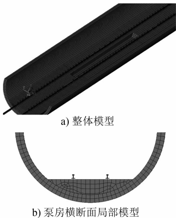
图 1 盾构隧道区间内置式泵房轨道结构模型 Fig. 1 Track structure model of built-in pump house in shield tunnel interval
