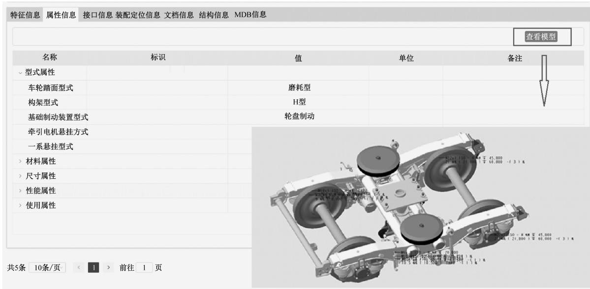
图 3 A 型地铁车辆转向架快速定制设计方案效果图截图 Fig. 3 Screenshot of a rapid customized design scheme for type A metro vehicle bogie
