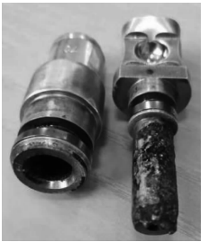
图1 电连接器插孔、插针(已烧损)实物图 Fig.1 Picture of the actual electrical connector socket and pin (burnt)
