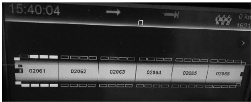
图 7 车门通信异常时的列车 HMI 截图 Fig. 7 Screenshot of train HMI in abnormal train door communication
