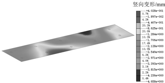
图 8 基坑土体开挖完成后高架桥面板竖向变形云图 Fig. 8 Vertical deformation nephogram of the viaduct bridge panel after completing foundation pit soil excavation
