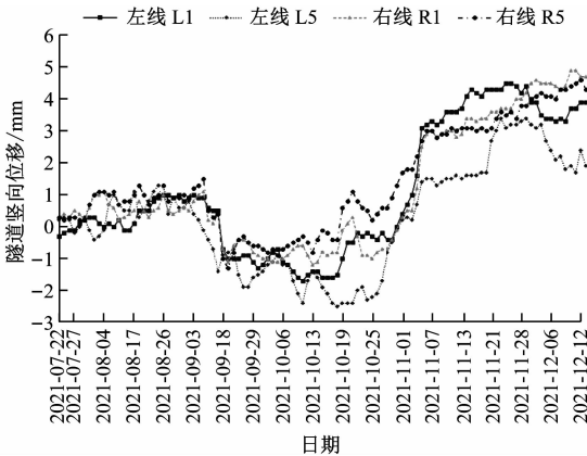
图 17 左右线的 DBC-13-01 与 DBC-13-05 监测点最大累计竖向位移 Fig. 17 Maximum cumulative deformation at monitoring points DBC-13-01 and DBC-13-05 on the left and right lines
