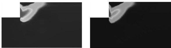
a) 1-1 断面处 b) 2-2 断面处 图 6 冷冻法施工前 2 个断面处的地层塑性区 Fig. 6 Stratum plastic zone at 2 sections before freezing method construction
