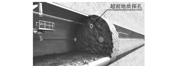
图 7 海底区间隧道矿山法施工的超前地质探孔布置示意图 Fig. 7 Diagram of advanced geological exploration hole layout for mining method construction of undersea section interval tunnel
