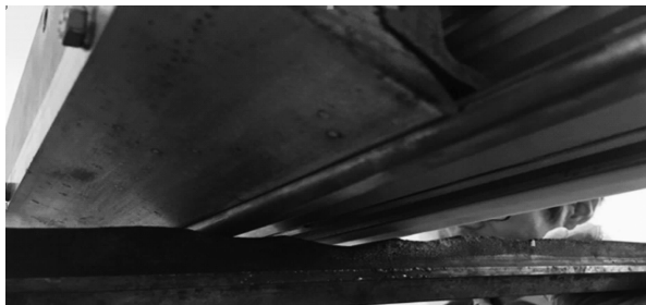
图3 碳滑板3个凹槽的间距与膨胀元件3条线的间距相符 Fig. 3 Spacing between the three grooves of carbon strip matching that between the 3 lines of expansion element
