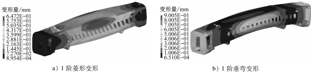
图 6 小窗户方案车体的模态振形 Fig.6 Modal shape of car body structure under small window scheme
