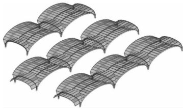
图 7 SAP 软件构建的新建钢屋盖模型 Fig.7 Newly-built steel roof model constructed by SAP software
