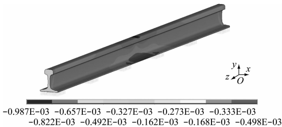
图3 静荷载为 200 kN 时钢轨沿 z 方向的应变云图 Fig. 3 Strain cloud diagram of the rail along the z direction under 200 kN static load
