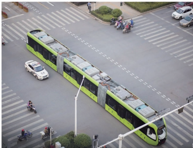
图 11 湖南株洲市的智轨系统 Fig. 11 Autonomous rapid rail transit (ART) in Zhuzhou, Hunan
