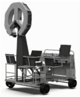
图 6 基于机器视觉的地铁隧道智能巡检设备 Fig. 6 Intelligent metro tunnel inspection equipment based on machine vision
