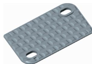
图 5 铁垫板下弹性垫板结构示意图 Fig. 5 Schematic diagram of the elastic pad structure under the iron plate
