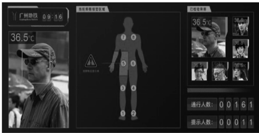
图 7 应用方式一的安检门液晶显示屏界面 Fig. 7 LCD screen interface of security inspection door in application mode I
